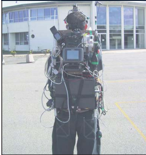
Figure 3. Tinmith outdoor backpack computer.
