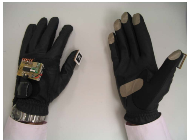
Figure 1 – The gloves shown from above and underneath. A custom controller board with an MSP430 and Promi-SD202 Bluetooth chip is used to interface with the gloves. Metallic fabric pads and conductive thread are used to detect finger presses. Fiducial markers are used for 3D tracking outdoors.
