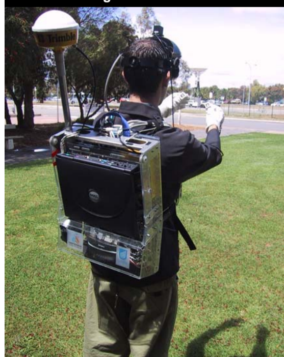
Fig 13 – The Tinmith-Endeavour 2002 backpack was properly manufactured and more refined, but was large and bulky in order to provide protection and flexibility for future change
