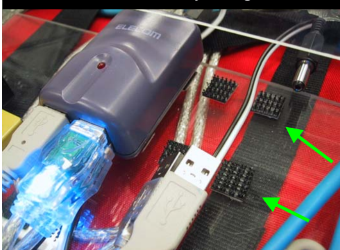
Fig 11 – Power distribution box, with DC-DC converters (at rear) to provide 5V, 6V, and 12V on varying plug sizes. 5V plugs are provided to power the USB hubs, which feed power to all 5V devices.
