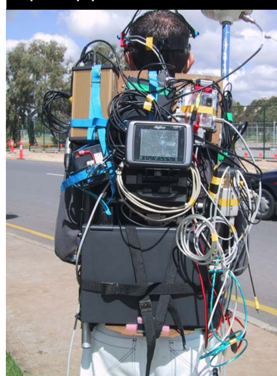
Fig 12 – The original Tinmith backpack was unorganised wires and components, with frequent equipment failure
