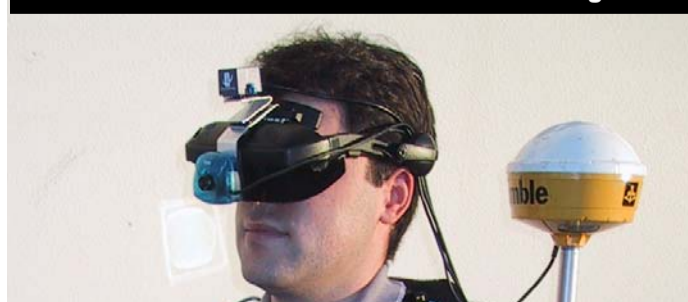
Fig 15 – IO-Glasses HMD, with InertiaCube 2 and PAL standard video camera for use with FPGA/MagicView
