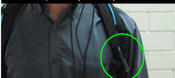
Fig 16 – Glove connectors are mounted onto the shoulder straps for easy access by the user
