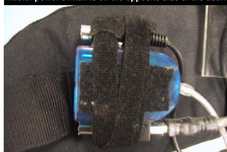
Fig 8 – External USB, HMD, and Firewire connectors are mounted on the waist straps for easy access. The master power switch is on the opposite side of the user.
