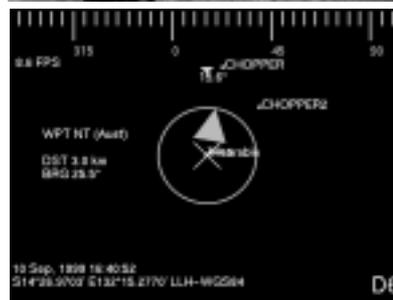
(b) God's-eye view, AR screen display superimposed on wearer's view. Note a helicopter (labelled CHOPPER) directly in front of the wearer, whose position is marked by an X.
