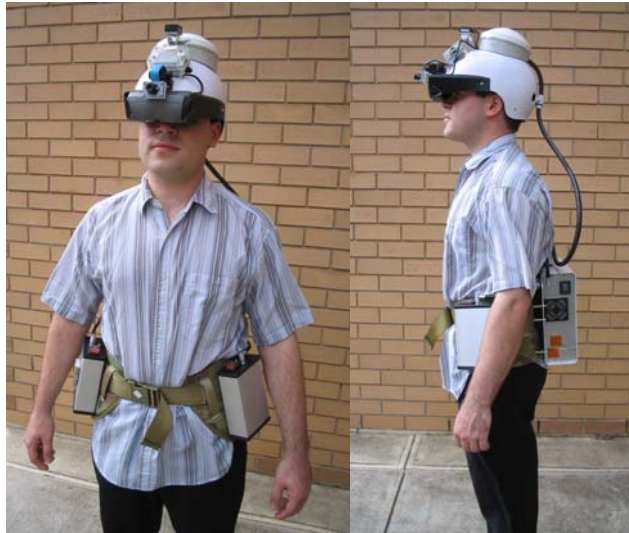
Figure 4 – User wearing the Tinmith 2005 mobile outdoor augmented reality system
