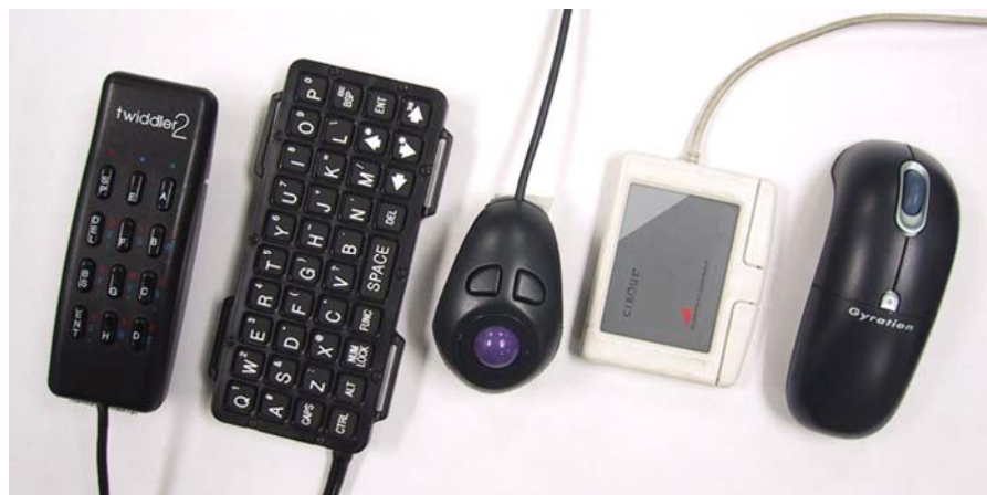
Figure 2-28 Wearable input devices suitable for use in outdoor environments (a) chordic keyboard, (b) forearm keyboard, (c) track-ball mouse, (d) touch-pad mouse, and (e) gyroscopic mouse
