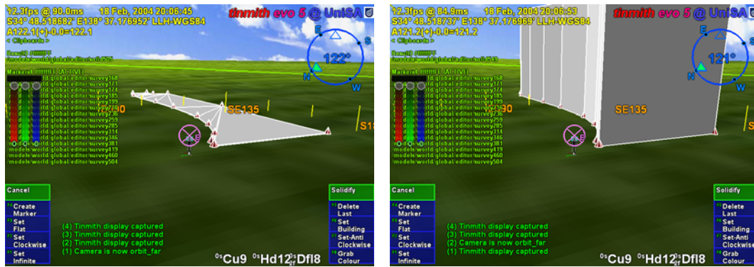
Figure 4-4 Example bread crumbs model extruded to form an unbounded solid shape
