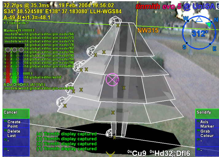
Figure 4-20 AR view of surface of revolution tree with markers on AR working plane
