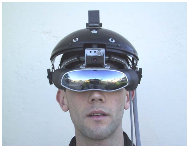
Figure 1-1 Example Sony Glasstron HMD with video camera and head tracker
