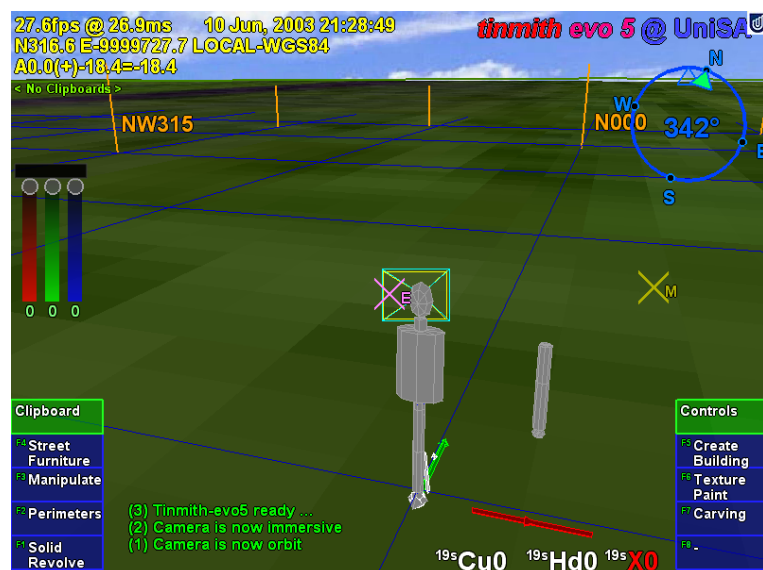
Figure 6-12 Distorted view of Tinmith-Metro showing improperly placed avatar objects when the resolution of OpenGL's internal values is exceeded
