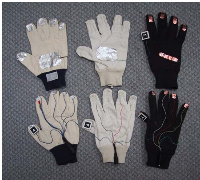
Figure 7-11 Designs of various versions of the glove and attached fiducial markers Shown are aluminium tape, wire wound, and copper tape designs
