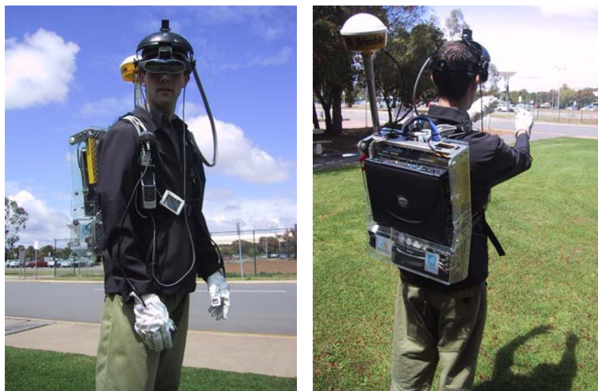
Figure 7-3 Front and rear views of the Tinmith-Endeavour backpack in use outdoors
