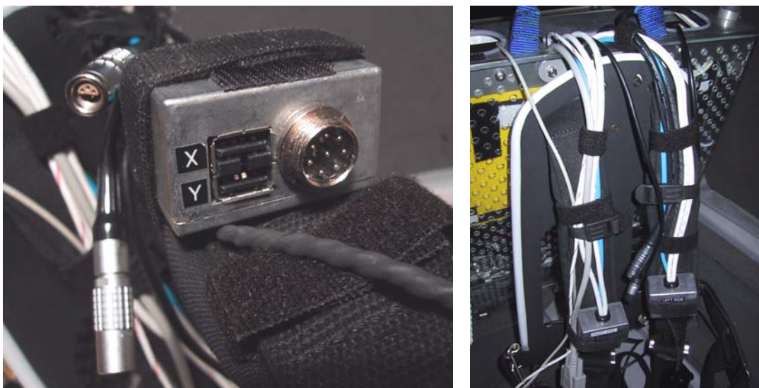
Figure 7-9 Two USB ports, glove connector, and cables mounted onto shoulder straps
