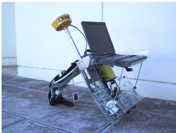
Figure 7-5 Backpack shown in desktop configuration, permitting normal use outside
