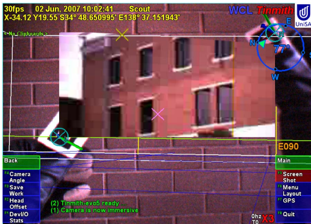
Figure 2 - Two handed magic-lens allows the user to see 'through' buildings
