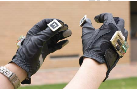
Fig. 11.6 Wireless pinch gloves allow the operation of menus using pinch gestures. The thumbs are tracked to provide 3D cursors for interaction
