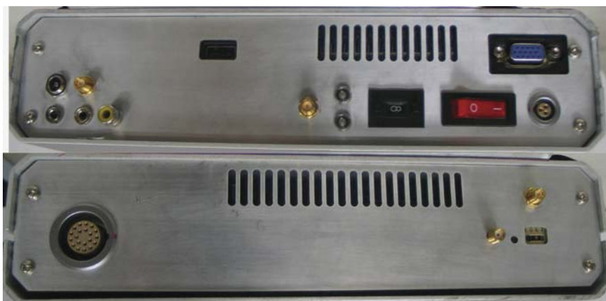
645 Fig. 11.9 Front and back panels of the main enclosure. A variety of connectors are available. 646 Integrated fan grills provide airflow for cooling
