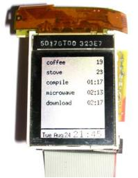
Figure 7. The timer application showing five different timers in operation.
