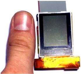
Figure 1 - Current watch prototype containing an LCD screen, MSP430 microcontroller, Bluetooth radio, and a temporary debugging cable.
