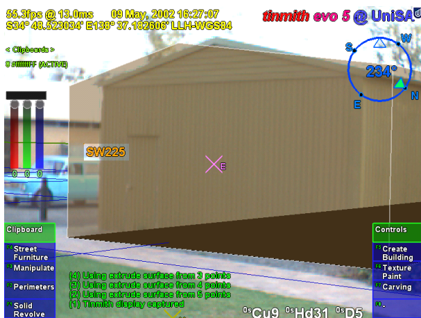
Plate 5 - Transparent 3D model captured using our construction at a distance techniques, overlaid onto the physical world building. This model uses both infinite carving planes and laser carving techniques
