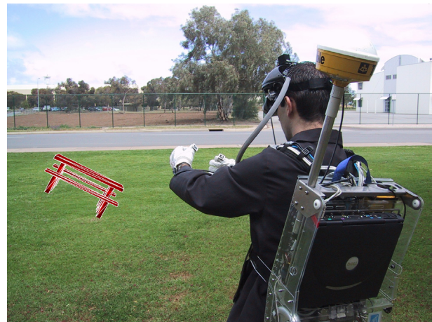
Plate 2 - Example interaction, showing a mobile augmented reality user performing a rotation operation on a virtual table at a distance, wearing the Tinmith-Endeavour backpack to provide real time AR
