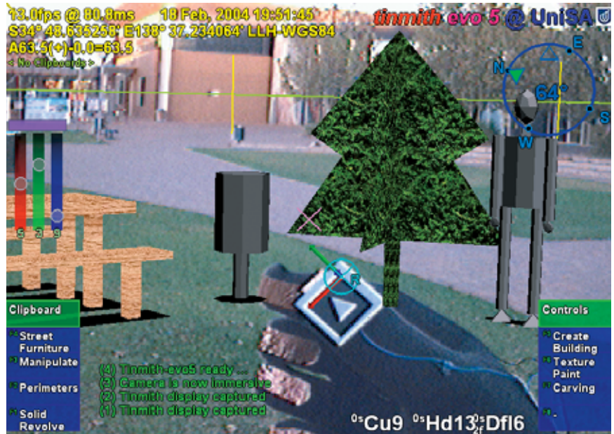
2 Users use tracked gloves to manipulate 3D objects against working planes. The blue and green menu strips show commands that can be selected by pressing the appropriate finger against the thumb on the gloves. Fiducial markers on the thumbs are tracked by the camera to provide pointing information to the user-interface software.
