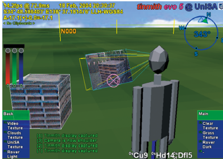
5 External viewpoint showing the user's body relative to other 3D objects. The live texture map shows what the user sees through the HMD, and that the system can automatically capture textures onto the surfaces of modeled objects.
