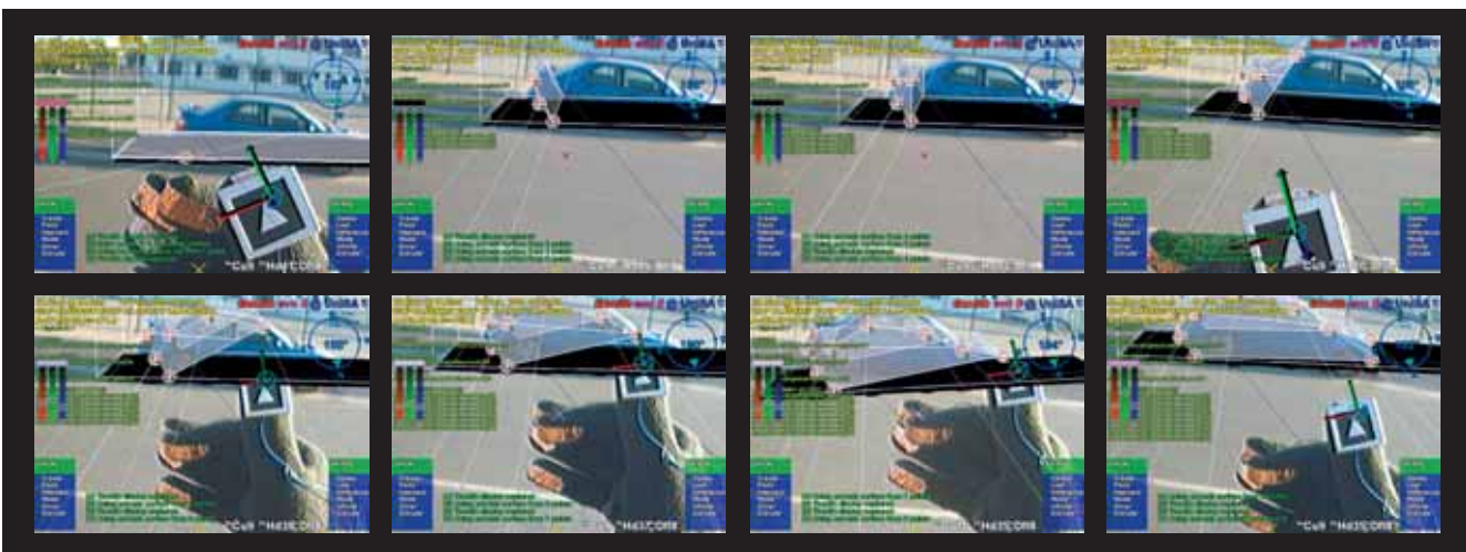
4 A user with tracked gloves carves out a solid box into the shape of an automobile.
