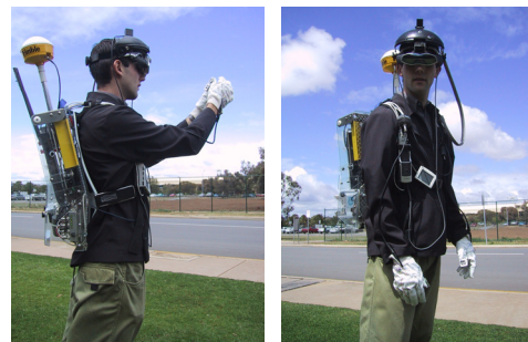
Figure 14 - The Tinmith Endeavour backpack, jointly developed by the authors at the Wearable Computer Lab of the University of South Australia with the Defence Science Technology Organisation - Salisbury
