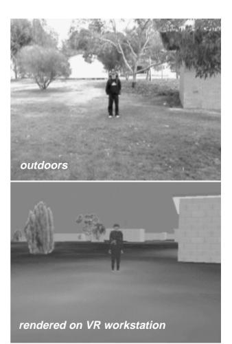
Figure 1. Linking a wearable AR system to a VR system enables mobile entities (the AR user, top) to be shown in relation to fixed entities (the trees and buildings) that exist in the terrain model, bottom.
