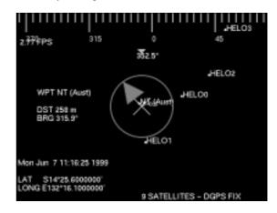
Figure 6. Two-dimensional, plan view of the battlefield, as generated to augment the user's outlook. Central cross marks the user location. Four helicopters, HELO0–HELO3, are shown as labelled dots in relation to the user's position.
