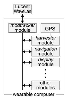
Figure 5. Software architecture of the wearable computer equipped to interact with ModSAF.
