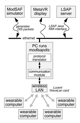
Figure 4. Block diagram of the combined AR/VR system. ModSAF generates a simulated battle environment, which is tracked in the LSAP database. One or more wearable computers in the field interact with the VR host PC via wireless network links. The entire engagement is visible on the MetaVR display.
