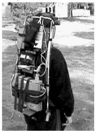
Figure 2. Photograph of the Tinmith-II wearable computer.
