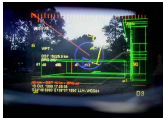
Figure 10 – AR Wireframe Building Overlay
