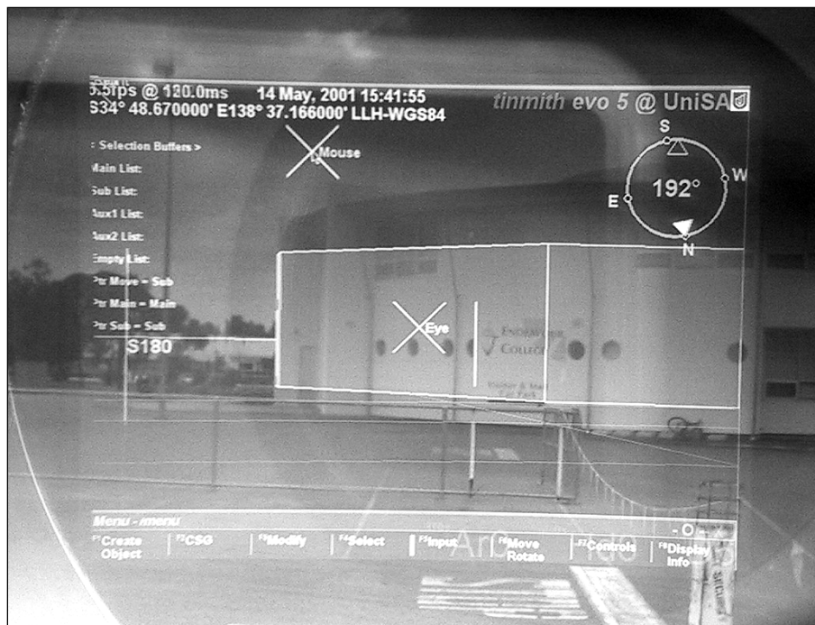
Figure 1 - Tinmith-Metro 3D building construction example, with user interface menu and situational awareness gadgets, demonstrating the Tinmith-evo5 architecture described in this paper
