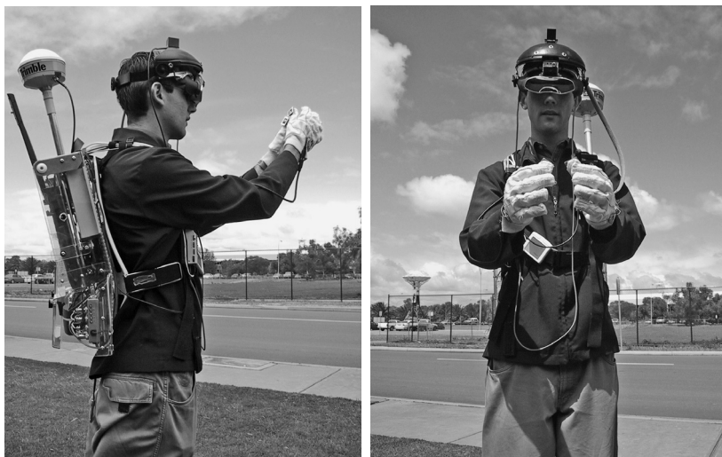
10.5 Tinmith-Endeavour outdoor augmented reality mobile computing system
